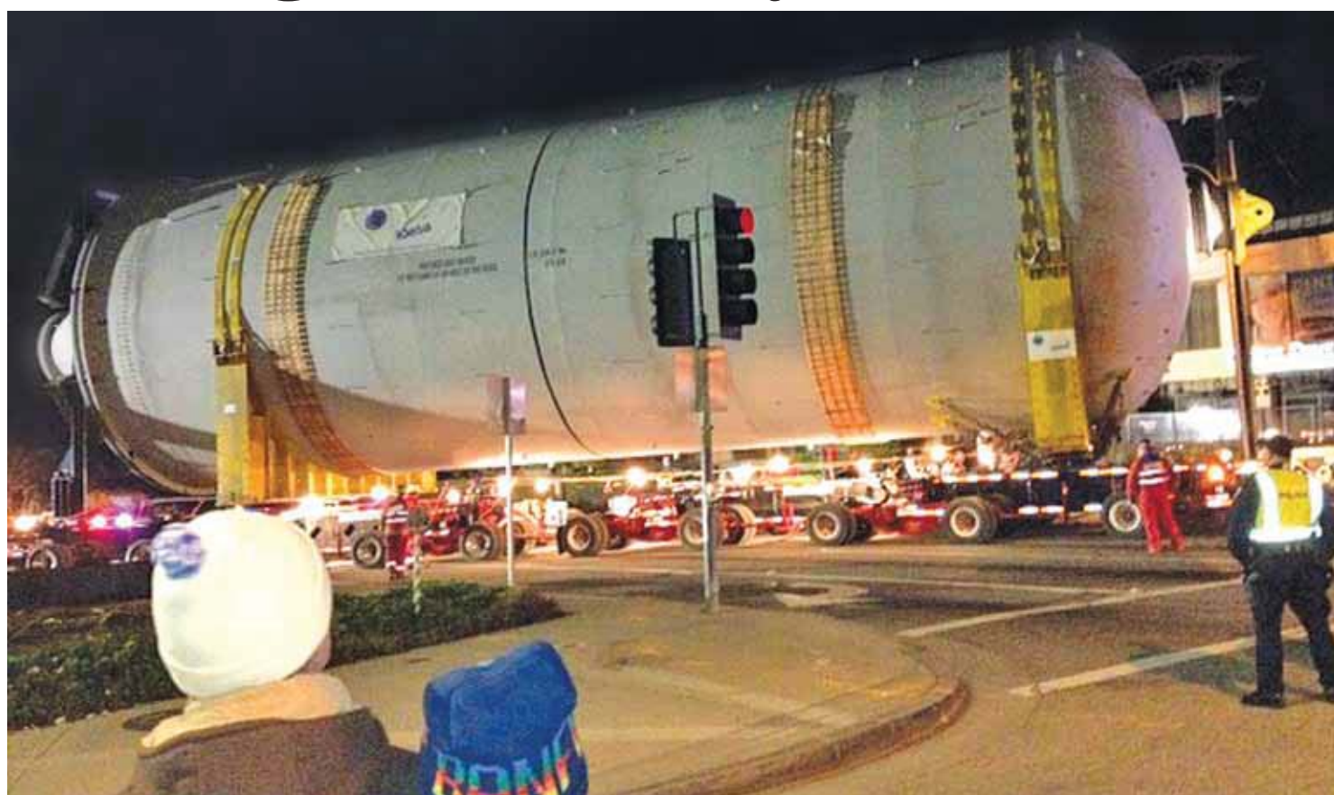
To clear the path for the refinery drums, Southern California Edison (SCE) crews turned the mast arms and street lights along Sepulveda Boulevard and on Rosecrans Avenue in Manhattan Beach, in preparation for the move of the first pair of drums, that were staged on SCE's lot at PCH and Herondo Street in Redondo Beach. Photo courtesy of Southern California Edison.
